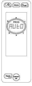
2- Press "ok" to confirm automatic programming activation. Press "reset" to go back to the starting page, namely to quit the function.
