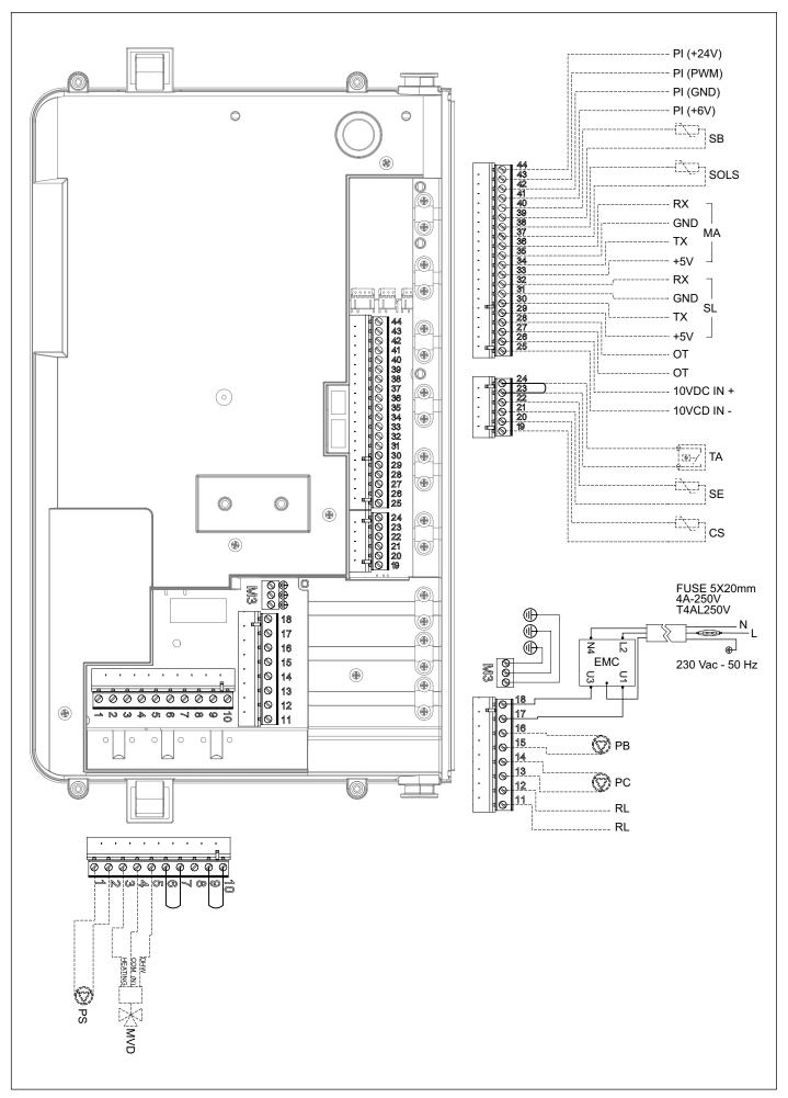
Fig. 29 Connections performed by the installer
