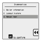
Press ok to start the MANUAL TEST function.
