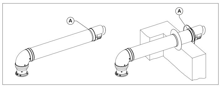
Fig. 15 Wall-mounted terminal installation
