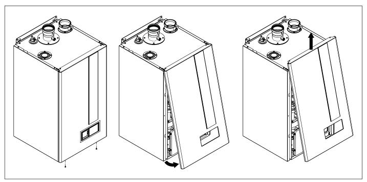
Fig. 26 Casing opening
