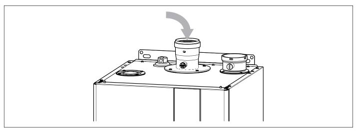
Fig. 37 Filling the trap
