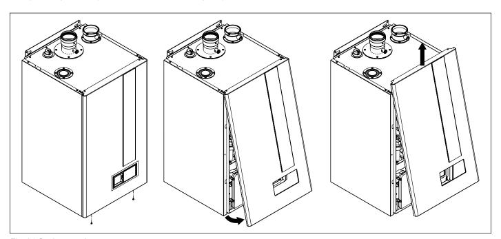
Fig. 31 Casing opening
