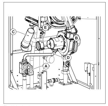
Fig. 32 Intake pipe
