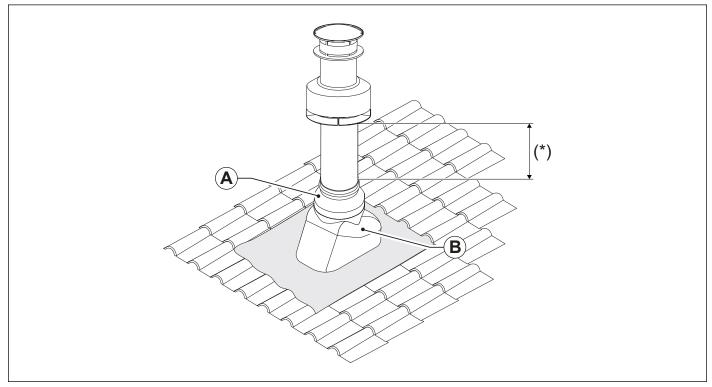
Fig. 17 Roof flue installation
