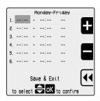
Press to go to the first slot end time setting.
