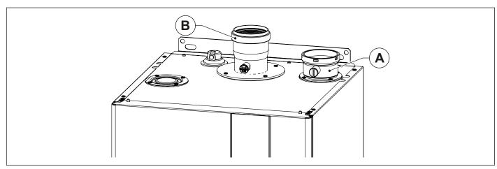
Fig. 18 Combustion analysis ports
