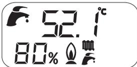
A rectangular display showing "52.1°C" in a large, black, digital font. Below it is "80%" followed by a small icon of a house with a flame and a radiator.
