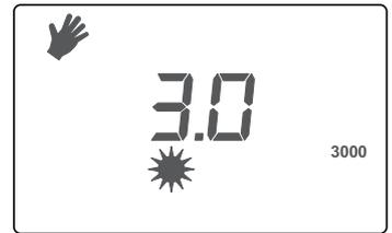
Turn knob clockwise to increase the temperature level; turn knob counter clockwise to decrease the temperature level. When you turn the knob, the temperature level value will flash. Press the knob to confirm the selected value or wait until the value stops flashing.
