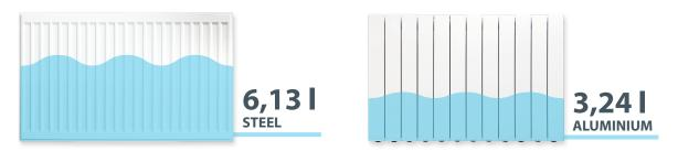
(Using a 500x1.000mm type 22 steel panel radiator as an example)
