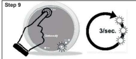
Press the **Rst** button again, the **Cloud** LED will blink fast three times every second; you are ready to pair the third Wi-Fi relay.
