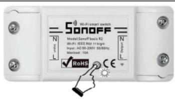
Now the relay is ready to be paired to the Gateway, fast click once on the relay button so that the relay is paired to the relevant Spot thermostat.
