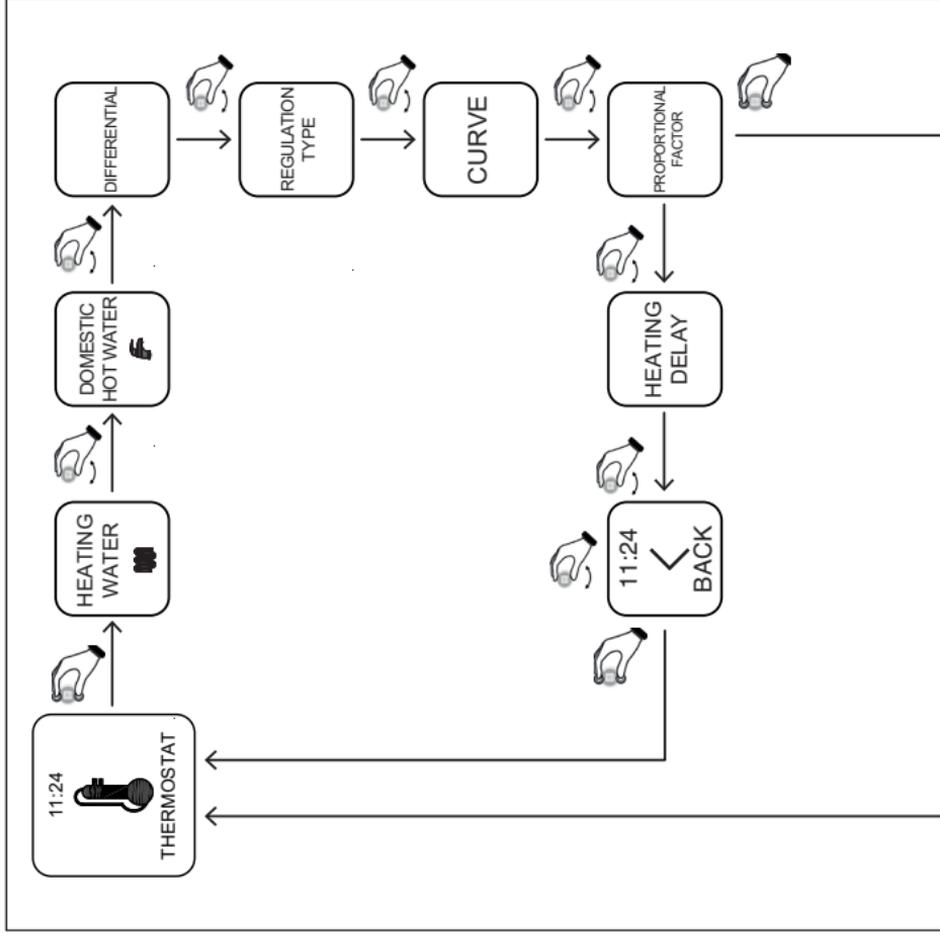
**PROPORTIONAL FACTOR:** this parameter affects the relation between external/ambient temperature and heating water temperature. The range goes from 0 to 20. The higher the value, the greater the influence of the external/ambient temperature. Recommended value: 8.
