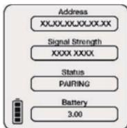
Press on the Spot thermostat again, the messages "PAIRING" and then "CONNECTED" will appear. Wait until "DISCONNECTED" appears. Spot is now paired to the Gateway.
