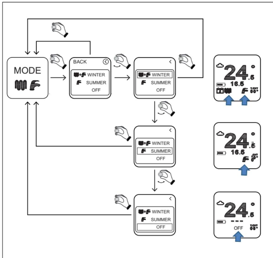
**WINTER:** the boiler is enabled to produce both hot water for heating and domestic hot water.
