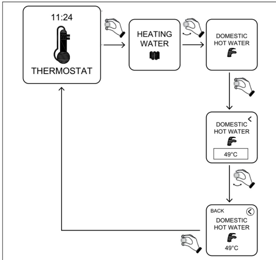
**DOMESTIC HOT WATER:** the boiler will produce domestic hot water at the temperature set with this parameter.
