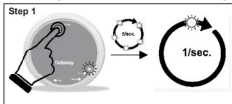
Press and hold the **Rst** button until you see the **BLE LED** switching from 5 fast blinks per second to one blink per second.
