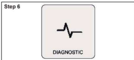
Press on the Spot thermostat in the main screen for three seconds until the "SCHEDULE" menu is shown, then rotate it until "SETTING" appears, confirm, rotate again until "DIAGNOSTIC" is shown and confirm.
