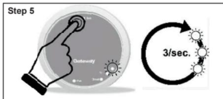
Press the Rst button again, the BLE LED will blink fast three times every second; you are ready to pair the third Spot thermostat.
