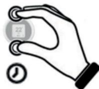
Press for a few seconds on the Spot thermostat until returning to the main menu.
