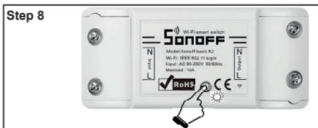
Now the relay is ready to be paired to the Gateway, fast click once on the relay button so that the relay is paired to the relevant Spot thermostat.
