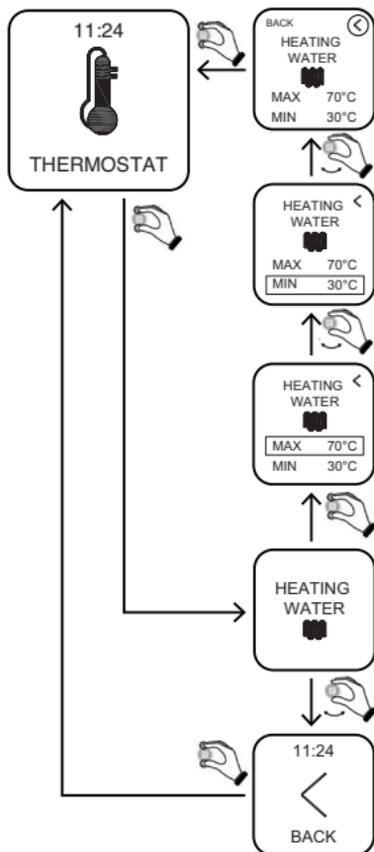
**MIN:** is the minimum temperature of the heating water that the boiler will provide in modulating operation
