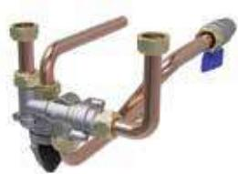
The Solar Kit for instant boilers allows you to bypass the boiler if water temperature from the solar tank is higher than 48 °C. It includes one unit integrating both a thermostatic deviating valve and an adjustable thermostatic mixing valve.
