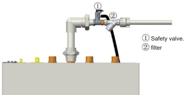
Installation method 1 for the drinking water safety valve (inlet water pressure = 0.1–0.5 MPa)
